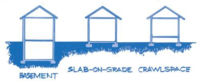
Radon reduction systems can be grouped by home foundation design. Find your type of foundation design above and read about which radon reduction systems may be best for your home.
